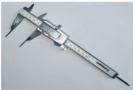
Figure 1. Modified digital Vernier caliper
